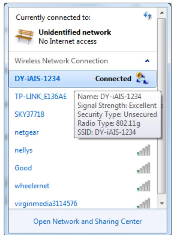
Once connected, run Tera Term and when the “New Connection” window is displayed, select the TelNet service, enter the IP address and Port number of the iAIS – which is always 169.254.1.1 Port 2000.
