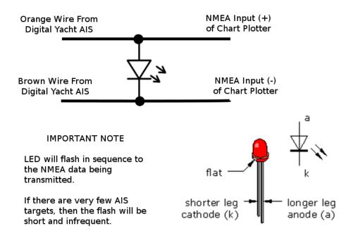
To test an NMEA0183 output, simple connect the LED across the NMEA + (A) and NMEA – (B) connections. In one direction the LED will not illuminate and in the other direction the LED should flash in time to the NMEA0183 data being received. No damage can be done to either the LED or the equipment being tested by connecting it the wrong way round.
