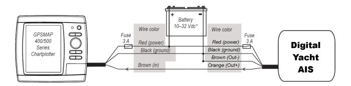
The following diagram is applicable to the Digital Yacht ANT200 Smart AIS antenna.
