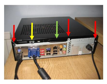
2. Placing your finger tips under the flap indicated by the green arrow, pull gently on the case until it slides away from the chassis by 10-15mm or until the case lid is clear of the silver flap with the hole in
