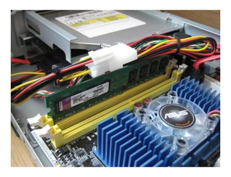
5. Being careful not to place to much downwards pressure on the motherboard or disturbing the cable assemblies passing close to the RAM modules, gently place a finger on one end of a RAM module and push down to make sure the RAM is properly seated in the socket. When the RAM is properly seated, the white plastic clip should fit neatly in the semi-circular cut-out of the RAM module – see image on next page. Repeat this step three more times, for each end of the two RAM modules.
