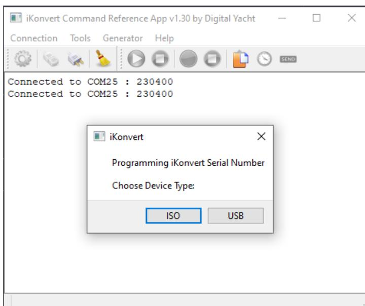
Select the relevant device type for the iKonvert you are using but clicking the “ISO” of “USB” button...
