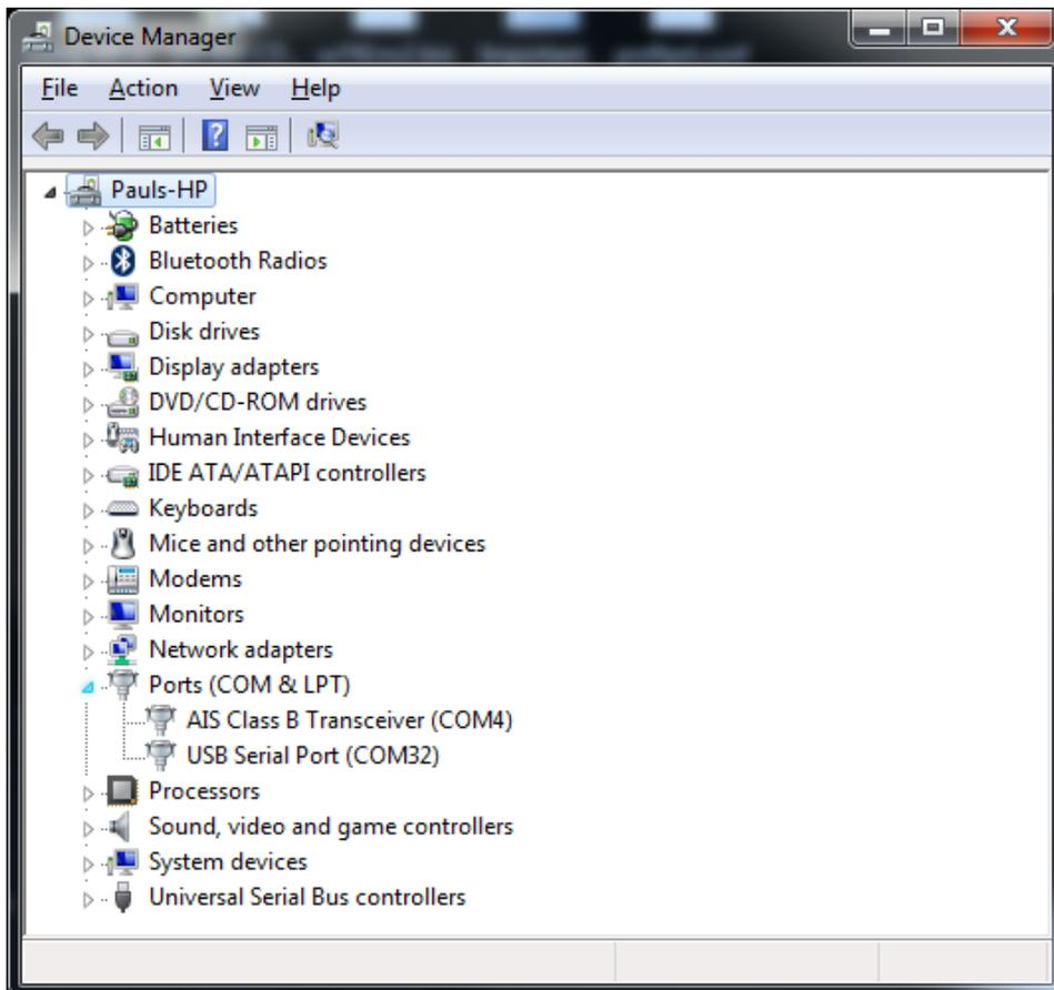
Apply power to the product, please note that no LEDs will illuminate in this Boot Loader mode, and run the STM Flash Loader Tool, which should see the window shown in Figure 1.
