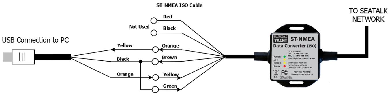
Plug the USB connector in to the Windows PC and as long as the PC is connected to the internet or it already has the USB driver loaded, it should allocate a COM port to the USB connection.
