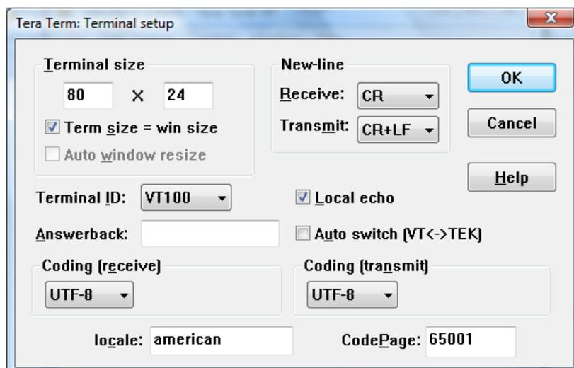
To change the configuration, you need to be in “Command” mode. To put the iAIS/WLN10/WLN10HS into “Command” mode, type \$\$\$ on your PC keyboard and then press the ENTER key. You should see the text CMD appear, just below the \*HELLO\* text, in the terminal window. Press the ENTER key again and a cursor will appear with the current software version shown.
