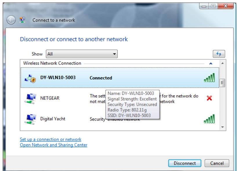
Once connected, run Tera Term and when the “New Connection” window is displayed, select the TelNet service, enter the IP address and Port number of our wireless device – which is 169.254.1.1 Port 2000.
