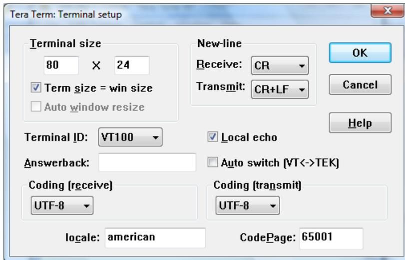
To change the configuration, you need to be in “Command” mode. To put our wireless device into “Command” mode, type **\$\$\$** on your PC keyboard and then press the ENTER key. You should see the text CMD appear, just below the \*HELLO\* text, in the terminal window. Press the ENTER key again and a cursor will appear with the current software version shown.
