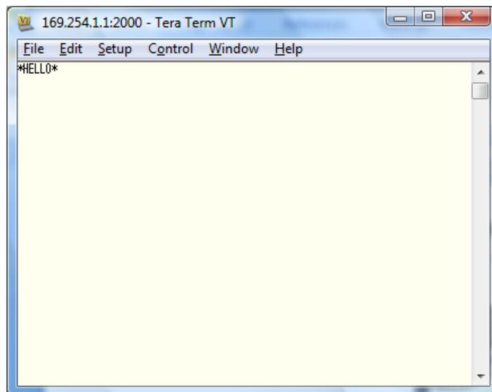
In order to see what you are typing in Tera Term, click on Setup>Terminal and then make sure the “Local Echo” option is ticked (see below). I also recommend setting the Transmit to “CR+LF” which will put a space between lines and make it easier to read the terminal screen. Once you have done this click “OK” to return to the terminal window.
