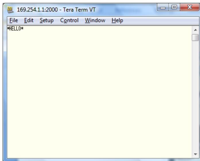
In order to see what you are typing in Tera Term, click on Setup>Terminal and then make sure the “Local Echo” option is ticked (see below). I also recommend setting the Transmit to “CR+LF” which will put a space between lines and make it easier to read the terminal screen. Once you have done this click “OK” to return to the terminal window.
