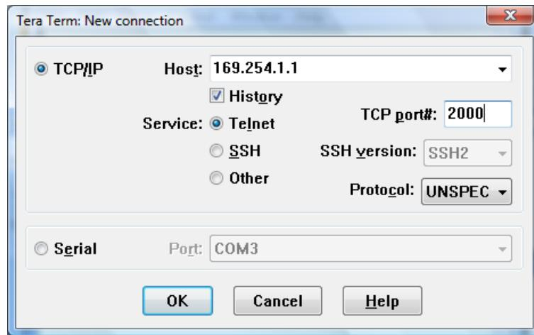
If Tera Term successfully creates a TCP/IP connection to our wireless device, then you should see the window below with the word “\*HELLO\*” displayed.
