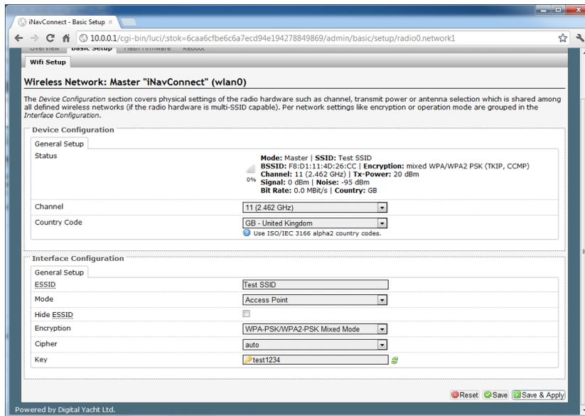
After setting the SSID, change the “Key” field to set the password. Click on the two green arrows icon to the right of this entry box to display the password that you have typed, rather than \*\*\*\*\*.
