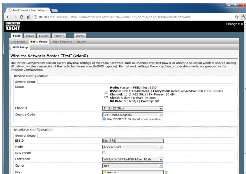
Changing the wireless password does not change the password you use to login to the iNavConnect web interface which will remain as "inavconnect".
