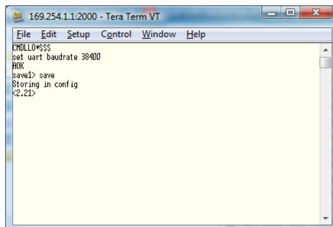
You can double check that the new setting has been accepted by typing **get uart** and then pressing the ENTER key, which will display the following information
