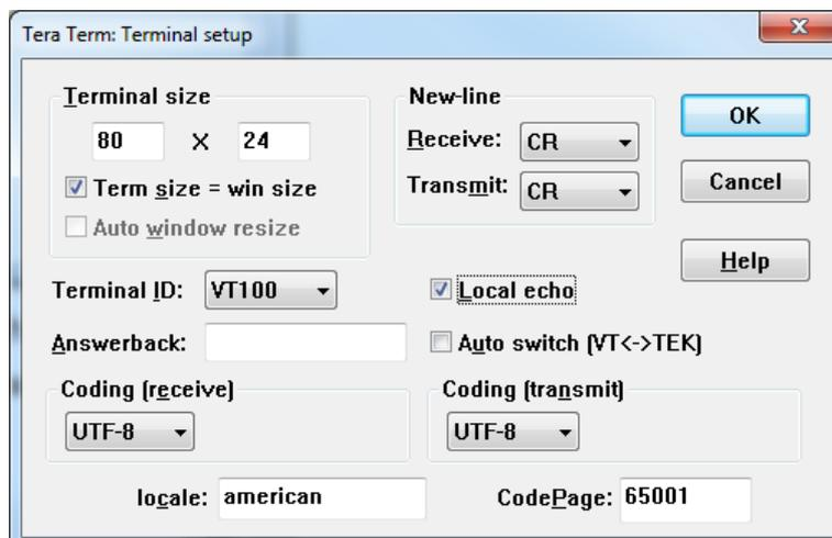
To place the WLN10/HS/Sonar Server in to Command Mode type three dollar signs \$\$\$ and then press the ENTER key. You should now see the following screen where the text CMD has been over typed on the
