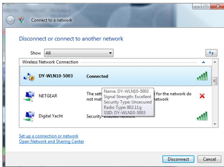
Once connected, run Tera Term and when the “New Connection” window is displayed enter the IP address and Port number of the WLN10/HS/Sonar Server – which is always 169.254.1.1 Port 2000.
