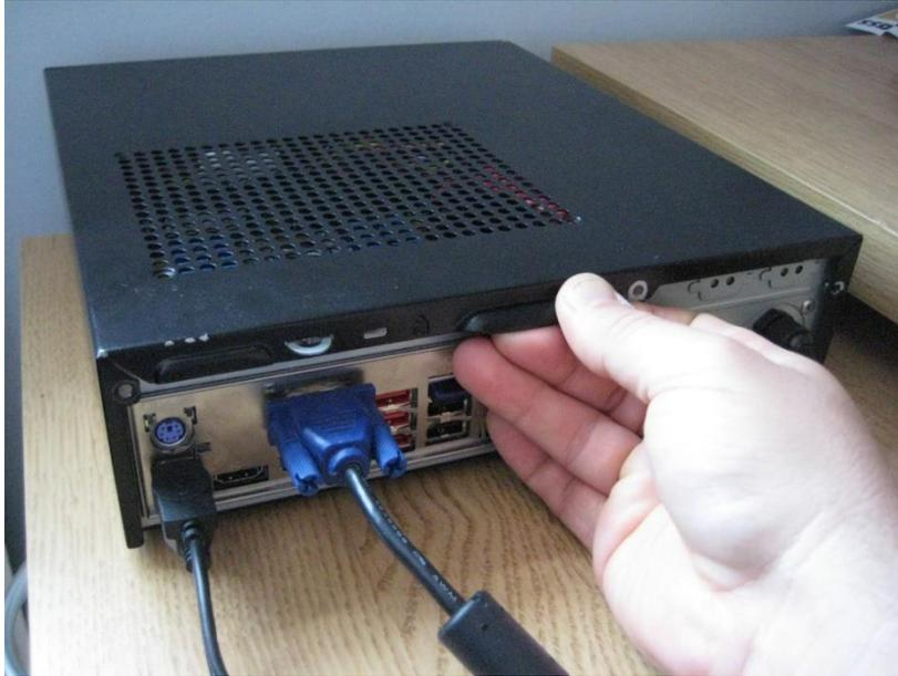
3. Once you have pulled back the case lid the required distance, it should be possible to gently lift the case lid off the chassis, revealing the AquaMedia motherboard and other components.
