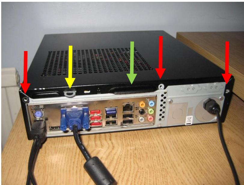
2. Placing your finger tips under the flap indicated by the green arrow, pull gently on the case until it slides away from the chassis by 10-15mm or until the case lid is clear of the silver flap with the hole in
