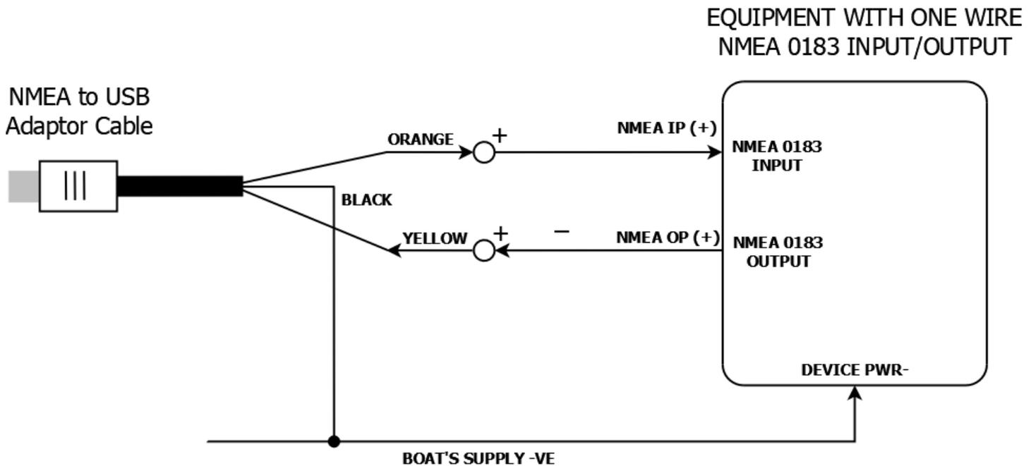
The two previous diagrams show how to wire the cable up for bi-directional communication, if you just want to receive data on to the computer, just wire up the Yellow and Black wires.
